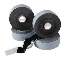
This product is made from a polyethylene carrier material, with butyl rubber adhesive applied on both sides. The inner butyl rubber layer is fully integrated with the outer layer, forming a continuous wrap-around coating.
