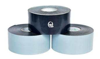
Our Polyethylene Seam Tape is a cold-applied tape designed for on-site anti-corrosion protection of circumferential welds on installed underground pipelines. It is composed of butyl rubber and polyethylene film, with an additional layer of anti-corrosion film. The tape is also highly adaptable and can be easily applied to elbows, fittings, and other complex shapes.
